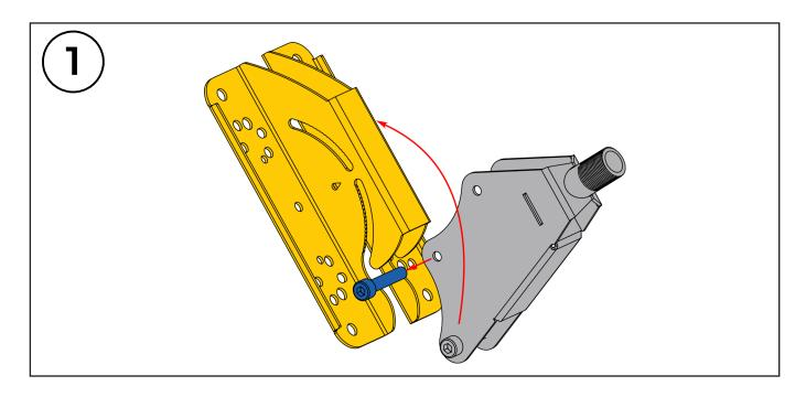
**1.** First, release the upper bolt which securing the speaker plate to the bracket. Now remove the speaker plate from the ceiling mount bracket.
