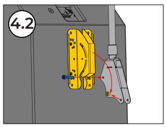
**4.2** Second position if you need an attachment angle from 45° to 90°. Move the screw to the second position on the ceiling mount bracket.
