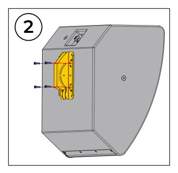
**2.** Screw the speaker plate to the rear (4) holes of the loudspeaker by using all (4) bolts.
