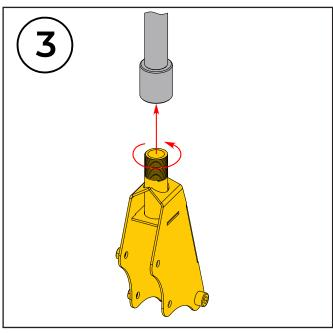
**3.** Install the ceiling mount bracket (screw) onto the distance tubes that was pre-installed.
