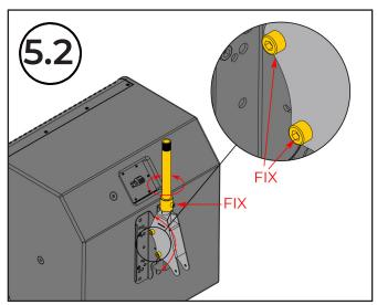
**5.2** Second position. Rotate the ceiling mount bracket in the distance tubes to the desired speaker position and secure the screw.
