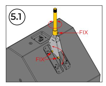
**5.1** First position. Rotate the ceiling mount bracket in the distance tubes to the desired speaker position and secure the screw.
