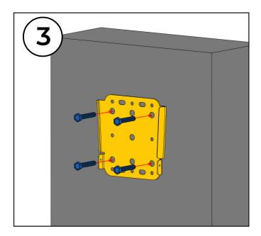
**3.** Screw the rear bracket to the wall surface by using a level and at least (4) fasteners. Use fasteners (4) that are suitable for the material your wall is made of.
