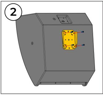
**1.** First, release the lower bolt which the front plate is attached to the rear bracket WMT-20. Now remove the front plate from the rear bracket.
