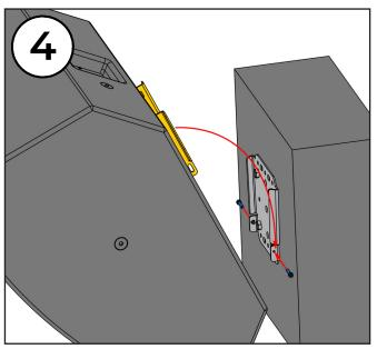
**4.** Slide the front plate along with the loudspeaker onto the rear bracket WMT-20. Then insert and tighten the lower bolts of the bracket.
